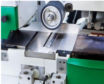
One driven roller in the machine table, hardened
